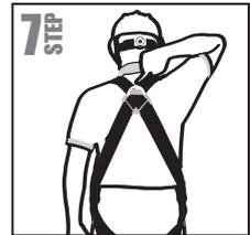
**Step 7 :** Use the back D-ring or the front as anchor point for fall arrest systems. To locate the anchor points on the harness, check for the "A" marking near them.
