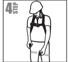
**Step 4 :** Pull the leg straps one by one around your thighs Outwards to your front as shown in Step 4.
