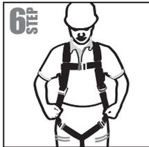
**Step 6 :** Tighten the leg straps by pulling the free ends of The straps until the harness fits perfectly to the body as shown in Step 6.
