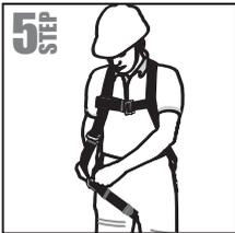
**Step 5 :** Close the buckles of the leg straps one by one as Shown in Step 5.
