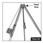
Winch is installed and now the tripod is ready for its claimed usage
