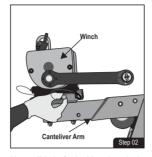
Use solid pin for locking the winch on pre-installed mounting bracket of Extreme Stainless Davit Arm.
