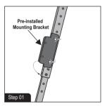
Locate the tripod leg that has preinstalled mounting bracket for installing the winch.
