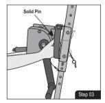
Use solid pin for locking the winch on pre-installed mounting bracket of tripod leg.
