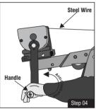
Pull out the handle of the winch outside and rotate it anti- clock wise to release the steel wire. Keep on releasing till you are able to release enough length such that it can pass over the pulleys of the Extreme Stainless Davit and get suspended vertically downwards.
