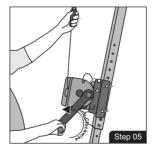
Pull out the handle of the winch outside and rotate it anti- clock wise to release the steel wire. Keep on releasing till you are able to release enough length such that it can pass over the pulleys of the tripod and get suspended vertically downwards.
